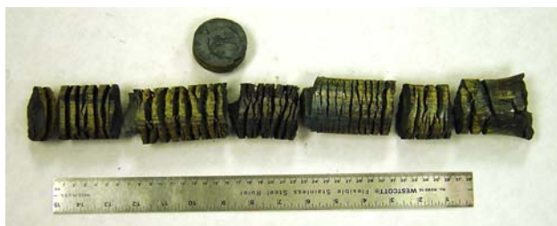
Fig. 1 Ni-40Ti-10Hf Extrusion attempt, unpublished research (Ref 5) at ATI Wah Chang
