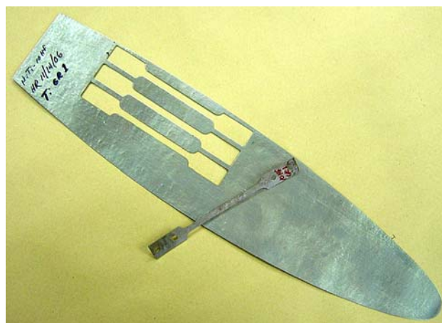
Fig. 3 Hot-rolled Ni-40Ti-10Hf sheet 0.6 mm thick showing CLD transformation test samples punched out at room temperature. Overall sample length is 16 \times 1.7 cm wide at grip section
